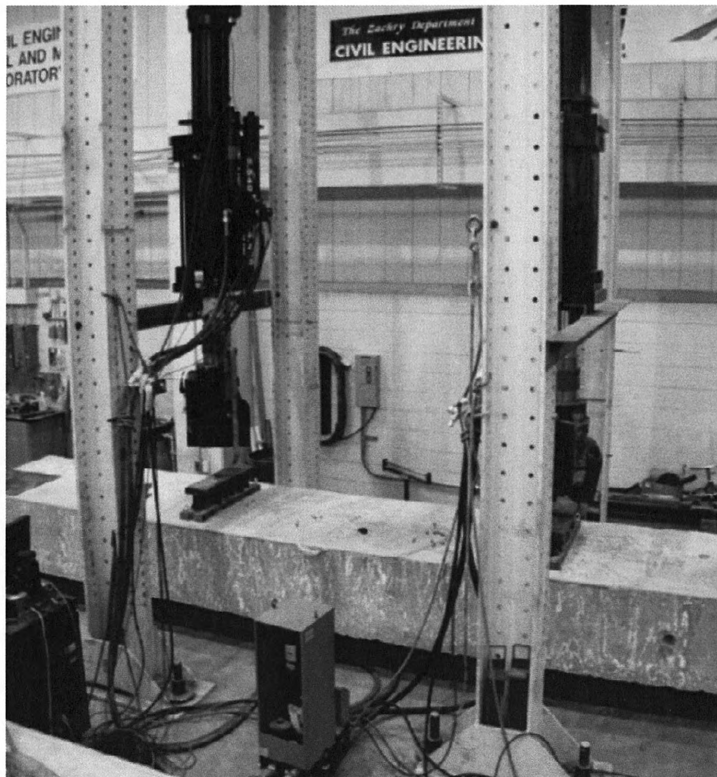
Figure 5-4. Specimen in the Four-Point Test Setup.
