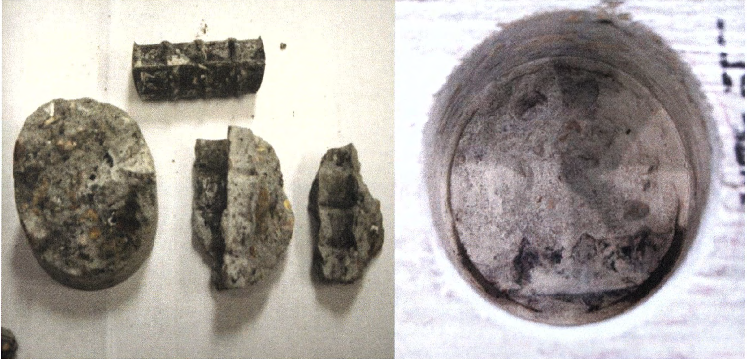
Figure 3-29. Core Extracted above Splice (left) and the Hole from that Core (right).
