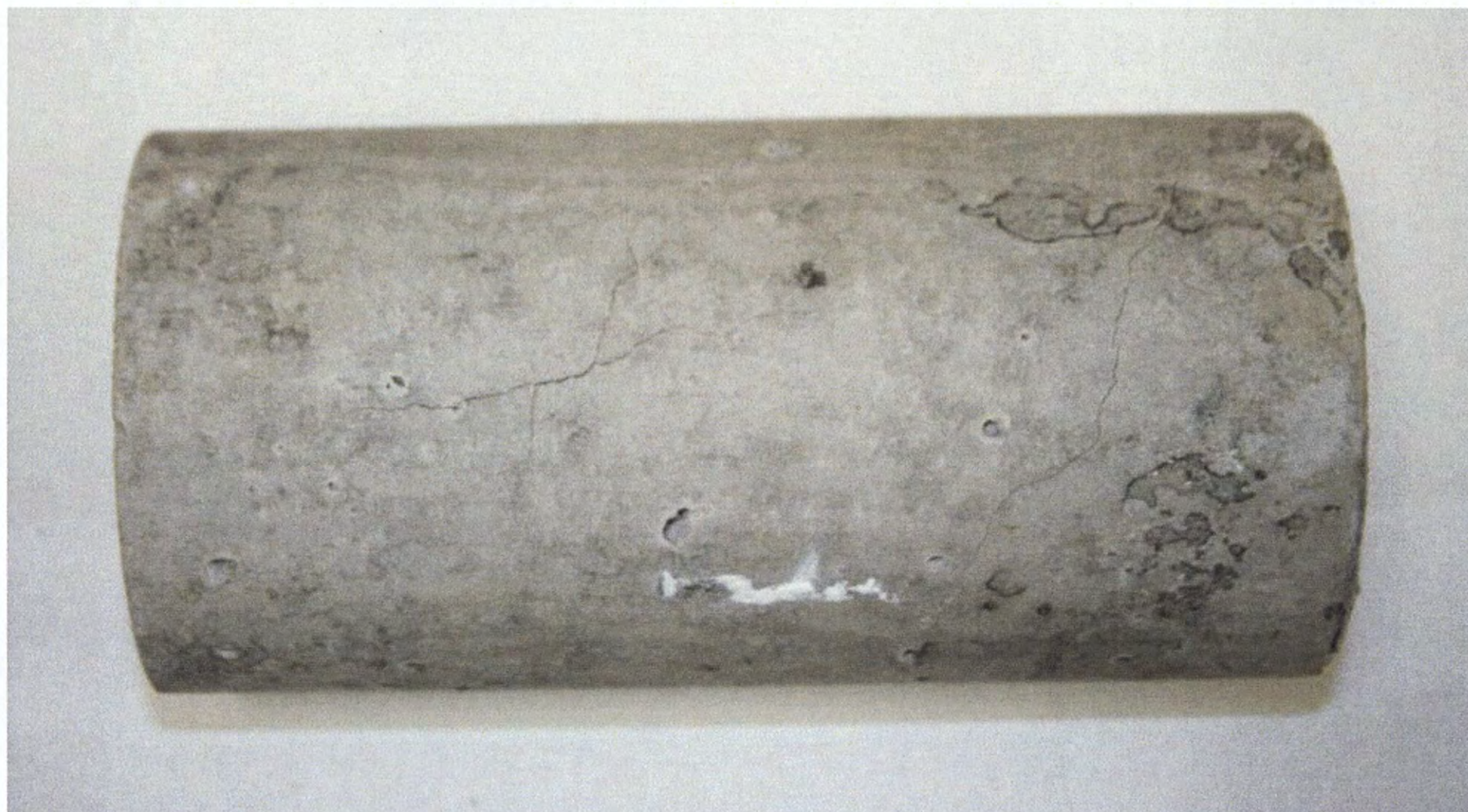
Figure 5-14. Cracking of a Cylinder Stored in the Curing Room.
