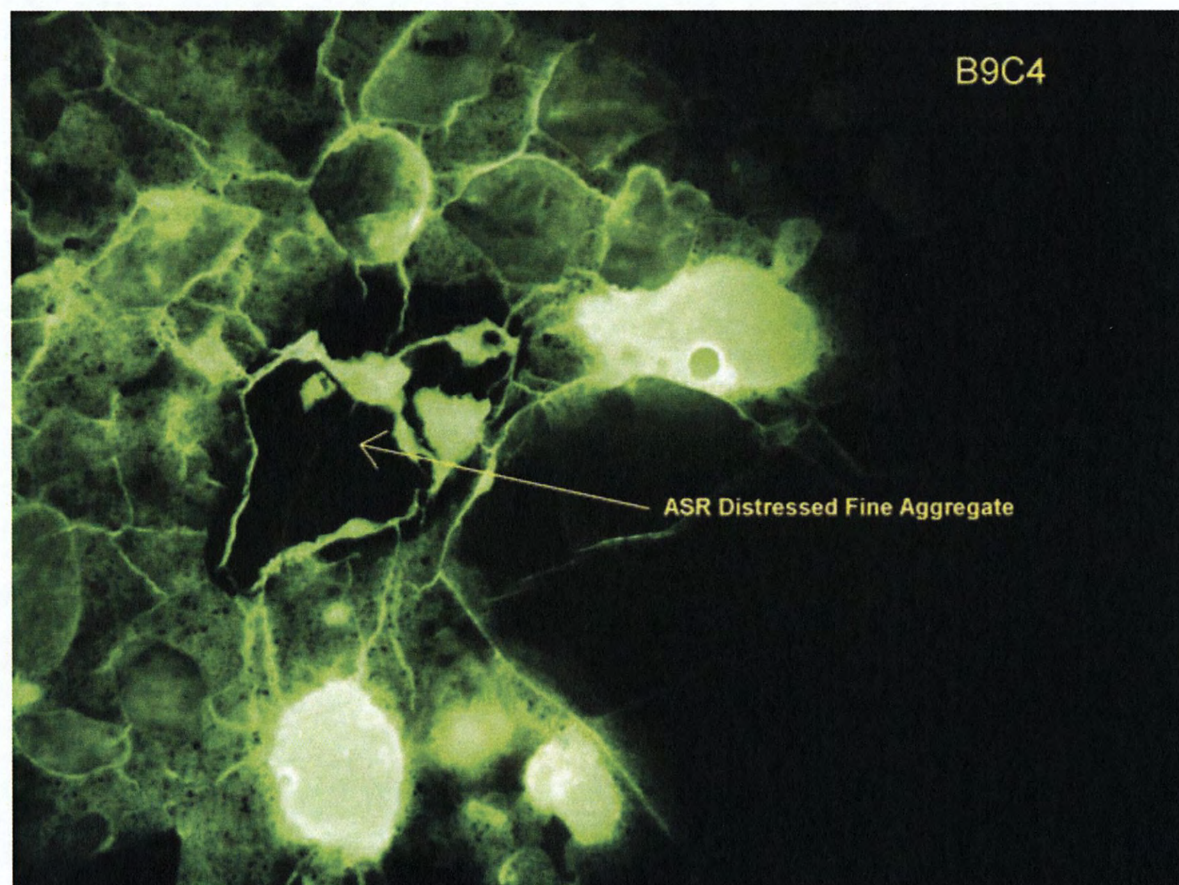
Fluorescent image illustrating distress associated with ASR reactive fine aggregate
