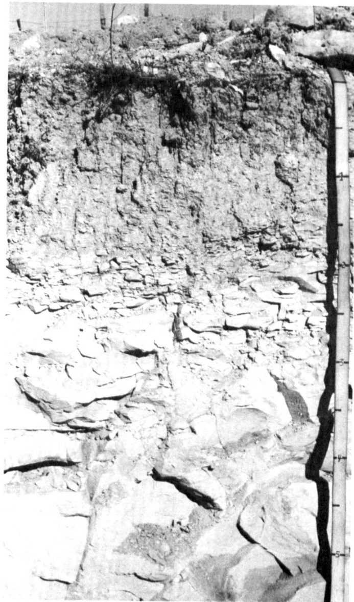
Figure 9.—Profile of Howe silty clay loam showing platy chalk fragments at a depth of about 20 inches and massive chalk below.
