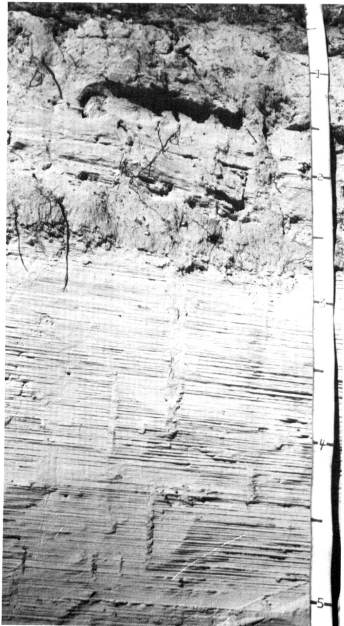
Figure 10.—Profile of Kiomatia fine sand. Continuous bedding planes are below a depth of about 30 inches.
